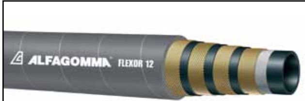
Four wire spiral - Flexor 12 Meets or exceeds SAE 100R12 - EN 856 R12 Meets flame resistance acceptance designation US MSHA IC-152/2
