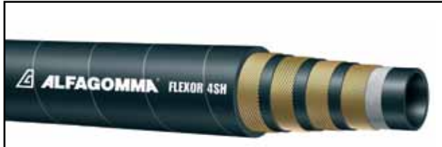
Four wire spiral - Flexor 4SH Meets or exceeds EN 856 4SH & ISO 3862 Meets flame resistance acceptance designation US MSHA IC-152/8
