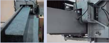
Integrated Y-Axis in Granite Table
