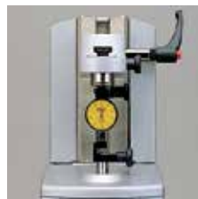
Using test indicator attachment set (02ASK000)
