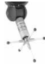
TP7 Probe (High-precision tough-trigger) See page L-20.
