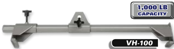
VH-100 Drum Lifter - Lifts from any angle. Load can be balanced. Easily adapted to lift objects of all shapes or lengths. Automatic "upsetting" of containers by adjusting sliding hoist collar. Holds rigidly even when load sways. Adjustment between jaws 16" minimum to 40" maximum. ■ Capacity 1,000 lbs. ■ Weight: 24 lbs.
