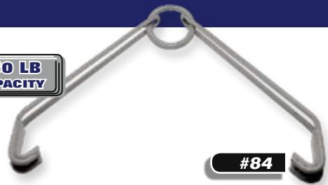
#84 Drum Sling - Lifts drum horizontally. The harder the pull, the tighter the grip on the drum. Use the drum sling to load your Pucel drum rack. ■ Capacity: 750 lbs. ■ Weight: 11 lbs.
