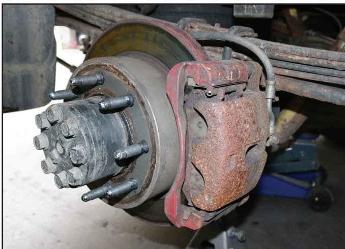
Caliper, after three years on the road, installed as purchased without any treatment
