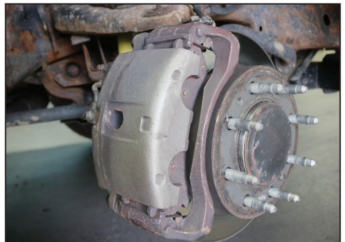
The same brand and part number of caliper as on the left, after the same three years, but sprayed with STEEL-IT Polyurethane Aerosol when installed
