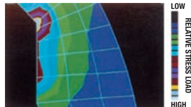
Conventional. This Finite Element Analysis display shows that ordinary sockets create extremely high stress loads at the fastener corner and at the socket's inside corners. The illustration shows that this stress is concentrated in a very small area.
