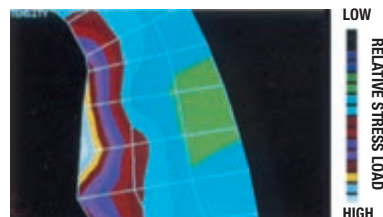
Wright Drive. The Wright Drive distributes stress evenly across the socket and fastener faces, away from the fastener corners, and over a larger flat contact area than ordinary sockets allow. There is a significant improvement in distribution of stress at the socket's inside surface.
